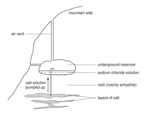
The salt is dissolved by water from underground springs and then pumped up to a reservoir where it is stored as a solution.
